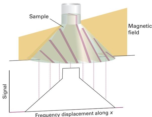
**Figure 1** In a magnetic field that varies linearly along the  $x$ -direction, the protons in different parts of an object (here a conical flask) resonate at different frequencies. The intensity at a particular frequency in the spectrum depends on the number of protons present at a particular value of  $x$ , and therefore the spectrum is an image of the proton distribution in the object.
