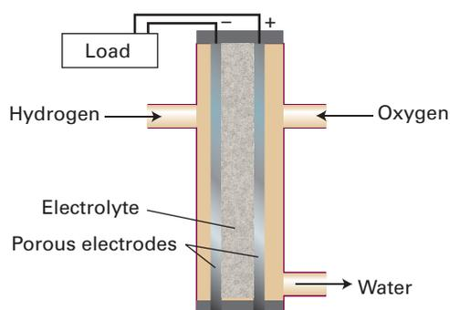
Figure 1 A single cell of a hydrogen/oxygen fuel cell. In practice, a stack of many cells is used.
